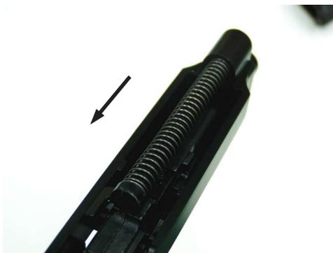
REMOVE THE RECOIL SPRING GUIDE AND SPRING.
