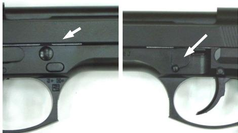
PRESS THE DISASSEMBLY LATCH RELEASE AND ROTATE THE DISASSEMBLY LATCH CLOCKWISE UNTIL IT STOPS.
