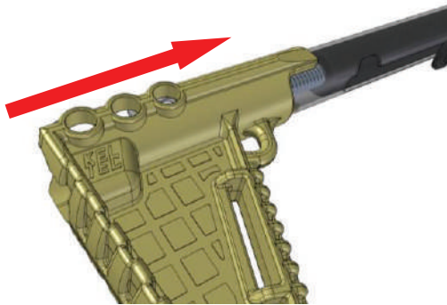
Figure E-4: Attaching the Stock
