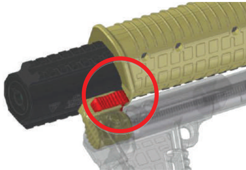
Figure C-7: Rotating Forend latching into the Latch Tab.
